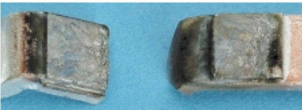
A contact just having reached a 'good worn in' level in an AC-3 application.
