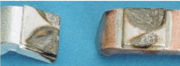
The appearance of contacts after a very low number of operation in an AC-3 application.
