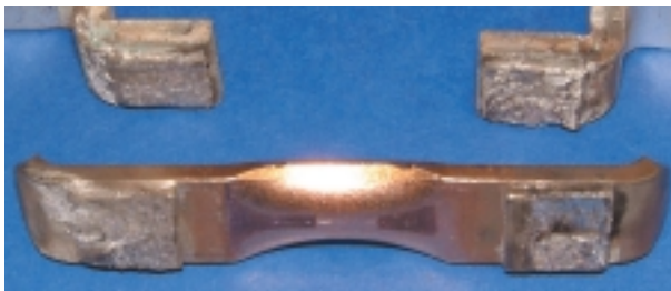
Early stage of fixed and movable contacts in an AC-3 application.
