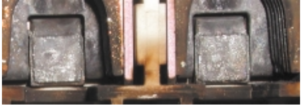
Early stage of fixed (above) and movable contacts (right), 5000 operations.
