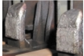
Mid-life stage of fixed (above) and movable contacts (right) 10000 operations.
