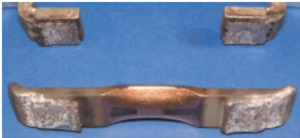
Mid-life stage of fixed and movable contacts in an AC-3 application
