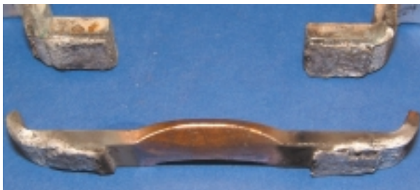
End of life of fixed and movable contacts in an AC-3 application
